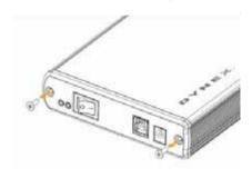
2 Remove the plastic end cap and circuit board.
