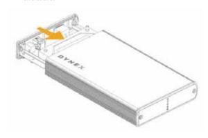
**5** Replace the two screws on the left-side panel.
