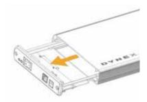
3 Connect your hard drive's SATA connector to the corresponding connector on the enclosure circuit board and secure the drive to the drive tray with the screws (4) provided.
