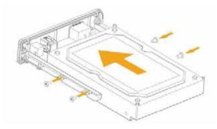
**4** Gently slide the drive tray, with drive attached, into the enclosure
